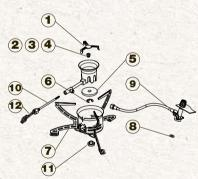
1: 731870 - Flame spreader 2: 730670 - Jet nipple 0.28 mm
