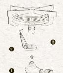
1: 732440 O-ring 2: 731840 Jet nipple 0.37 mm 3: 720120 Piezo igniter
